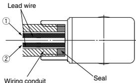
(Bore size G1/2 Tightening torque 0.5 to 0.6 N·m)
